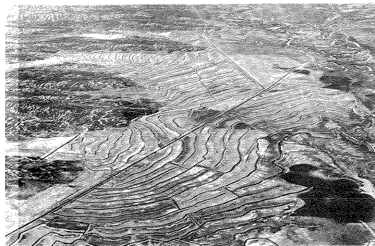
Waterspreading by means of contour dikes and ditches helps to slow runoff and give time for restoring vegetation.
