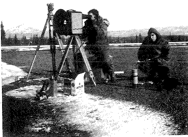
BLM surveyors set up their instruments on top of a school building to measure changes in the landscape.
